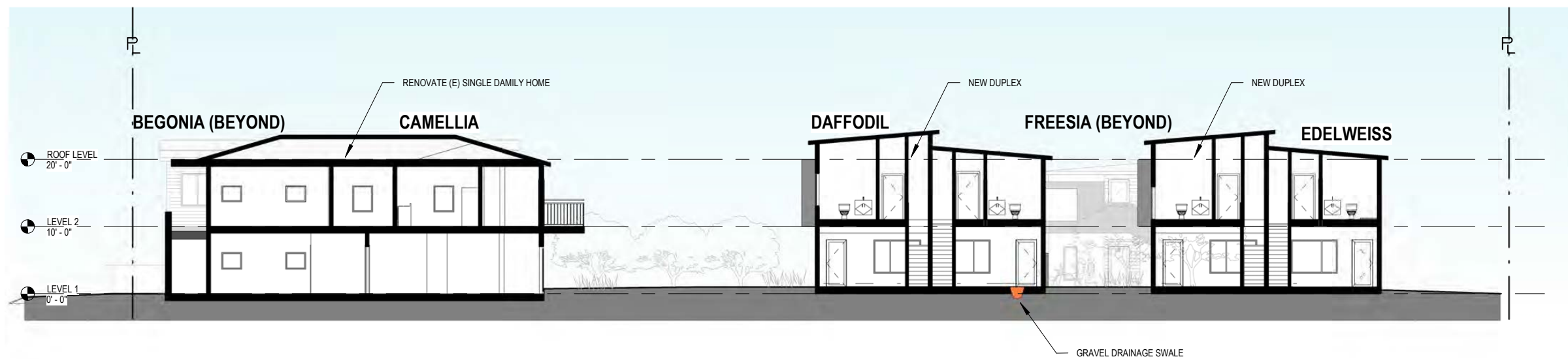
2 Building Section Looking West 1/16" = 1'-0"
